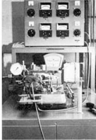
Rheology testing of compounds grades the flow characteristics
